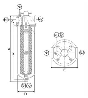
N1: Inlet, N2:Outlet, N3: Vent, N4: Drain
